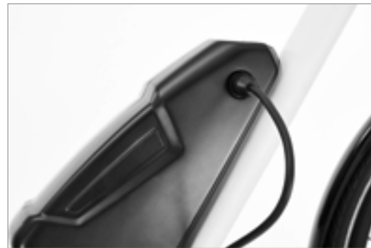
Charging the battery
