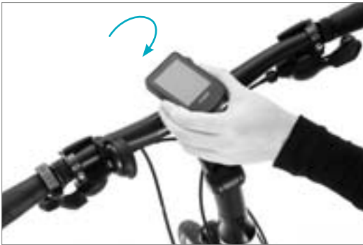
Mounting the display
