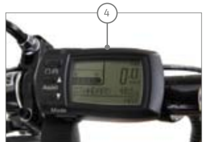
LCD control panel
