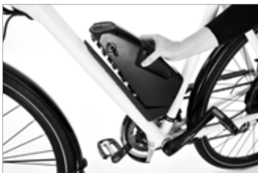
Installing the battery
