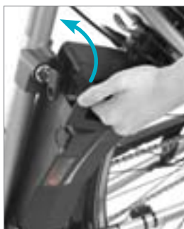
Reinstalling the battery
