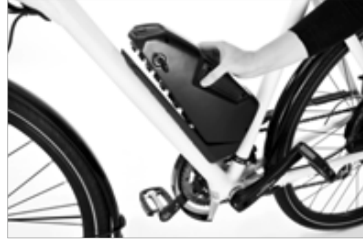
Installing the battery
