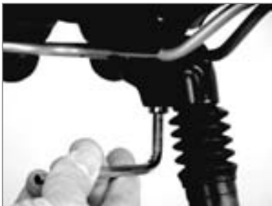
Adjusting the saddle angle
