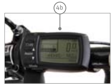
LCD control panel
