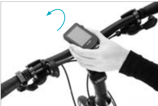
Removing the display
