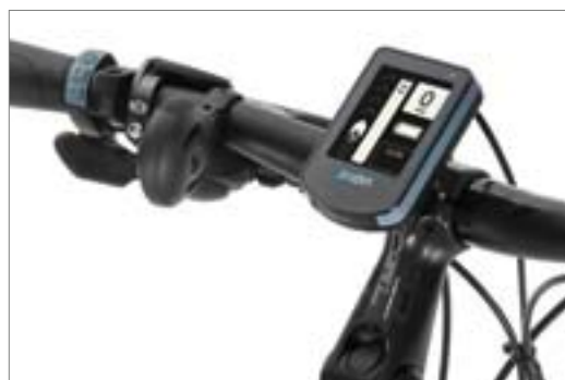
Control panel and display
