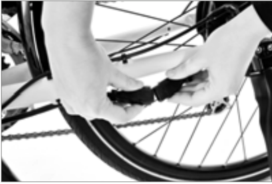
Disconnecting the cable
