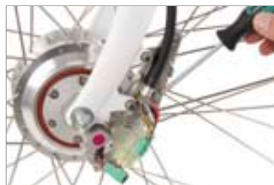
Base plate with cables and connectors
