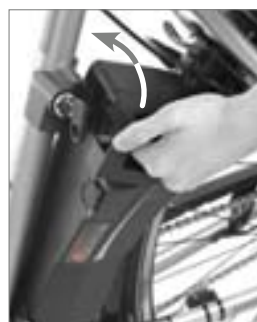
Reinstalling the battery
