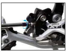
1. Loosen the B-tension adjustment screw.
