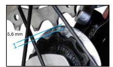
2. Then turn the B-tension adjustment screw to adjust the G-G distance so that the distance between the guide pulley and the sprocket is 5 – 6 mm. (Picture without chain for greater clarity).
