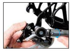
While keeping the rear derailleur in the correct position, tighten the bolt.
