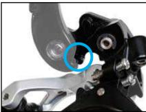
Periodically check that there is no gap between the dropout and the bracket, as this could cause problems with gear shifting performance.
