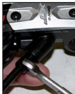
3. Unscrew the connecting bolt and remove the line from the lever.
