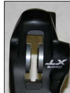
2. Squeeze the lever a few times to extract the pistons. Do not let the pistons come completely out of the cali- per.
