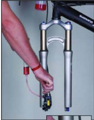
11. Close the bleed nipple (4-6nm; 35-53 in. lbs.).
