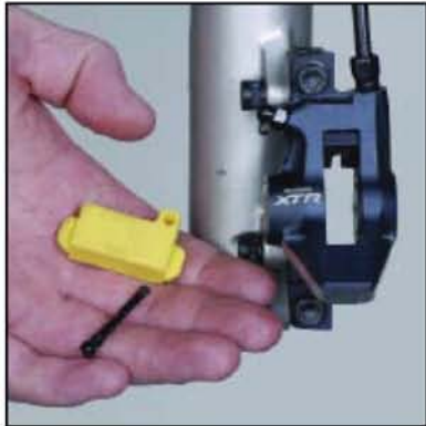
13. Once the lever feels firm, remove the yellow bleeding block from the caliper.
