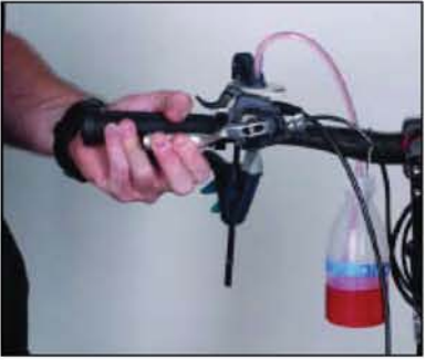
9. Once no more bubbles appear at the reservoir, stop pressure on the syringe. Close the bleed nipple and cycle the brake 5-10 times. More bubbles will make their way from the reservoir into the transparent tube and catch bottle.
