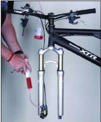
8. While pushing mineral oil through the system, be sure that all excess oil is flowing in to the plastic catch bottle attached to reservoir. Continue to push fluid through system until no bubbles appear in the reservoir.
