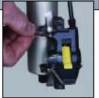
11. Close the bleed nipple (4-6nm; 35-53 in. lbs.).
